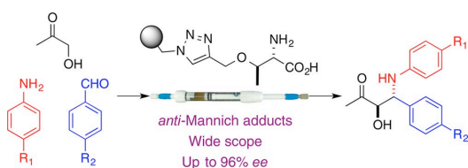
Fig. 1 – Continuous Flow Enantioselective Three-Component anti -Mannich Reactions Catalyzed by a Polymer-Supported Threonine Derivative.
